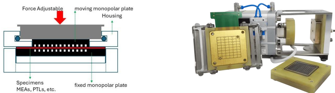
Figure 2: Function principle of the quick Connect Fixture cell frame and pressure transmission from the pneumatic cylinder to the cell area.
