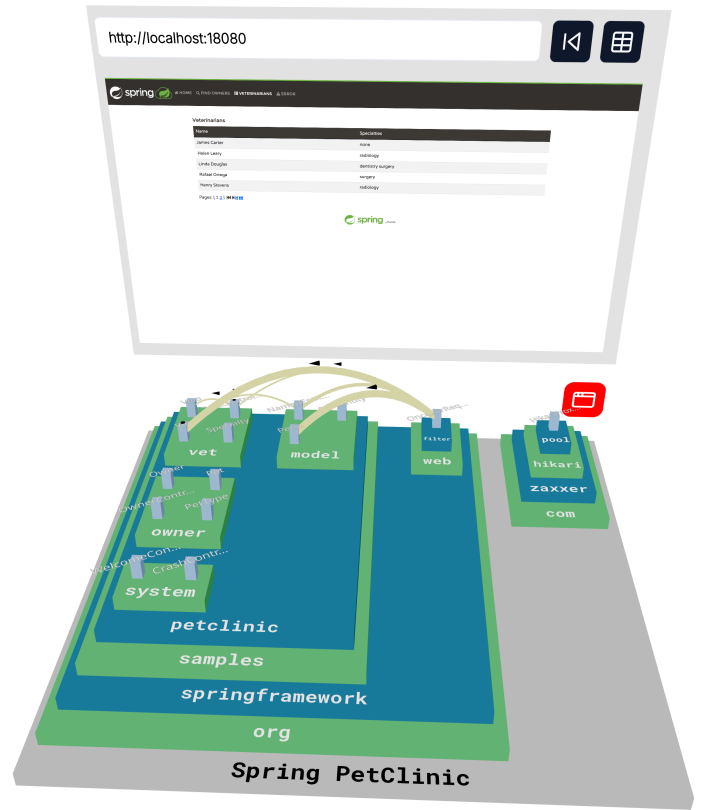
Fig. 1: Software city of the dynamically instrumented PetClinic with opened embedded browser. User input on the embedded iframe leads to the generation of trace data which is reflected in the software city.
