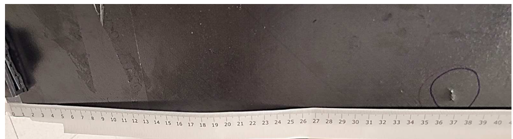
Figure 15. Detail of the flaw onset on the element and distance from the initial edge.
