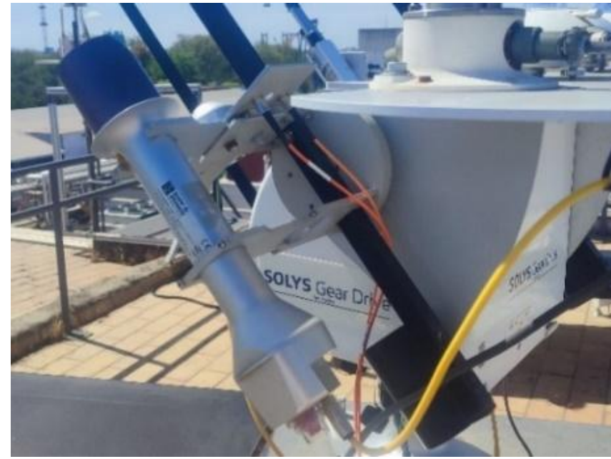
Mounting of the fibers onto the solar tracker and placed next to a commercial pyrheliometer
