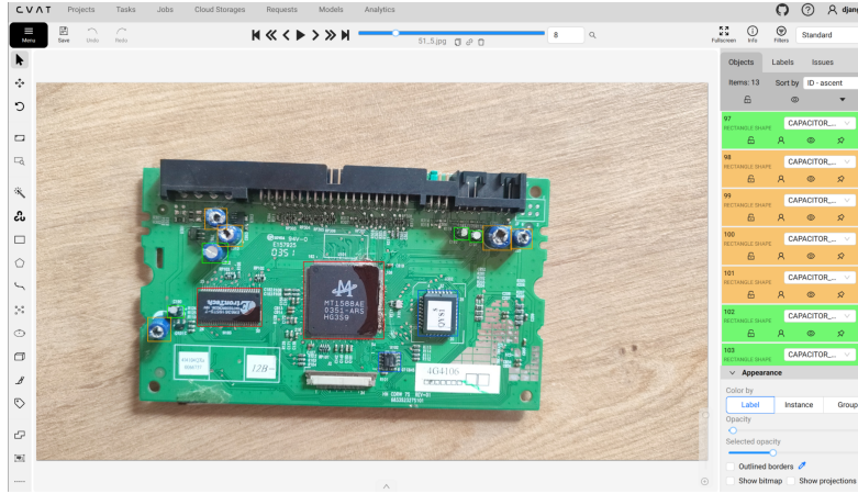
Fig. 5: Example of image annotations in CVAT. Bounding boxes are drawn around ICs and capacitors and labeled as either defective or non-defective.
