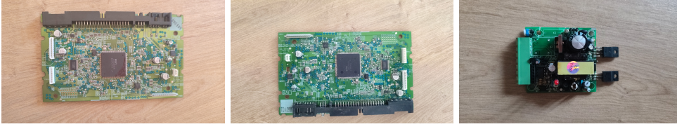
Fig. 1: Examples of defect types included in the dataset. Left: IC with burn marks; Middle: IC with dismantled pins; Right: Popped capacitor.
