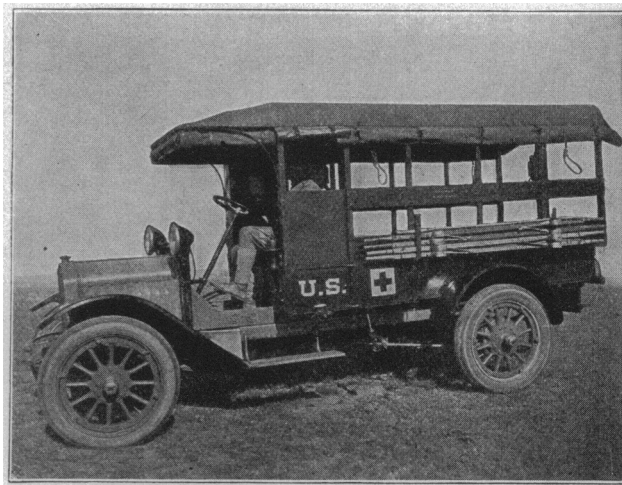
Fig. 6.—Type of motor ambulance being furnished to army; mounted on General Motors, Buick or Service truck chassis; it carries four recumbent or eight sitting patients; the upper litters are supported by the strap slings shown in the photograph illustration.
