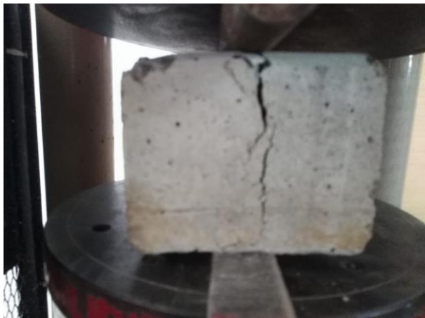
Figure 5. test setup used for tensile splitting strength tests
