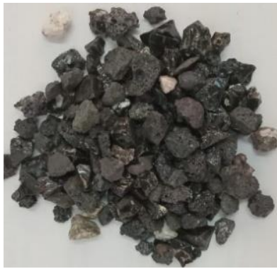
Figure 3. Sieve analysis results of separated coarse aggregates from waste steel slag and a photograph of separated coarse aggregates
