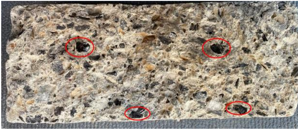
Figure 7. Photographs taken on failure plane of a sample with steel slag aggregates
