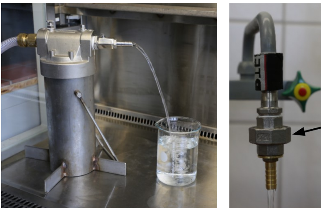
Figure SI.1: Demonstration of two quickly-constructed and mobile tap water filtration devices for the provision of ample MPF water as required for many tasks in a MP laboratory. (A) A stainless steel cartridge filter is used (pore size below the minimum MP size limit, here: 5 \mu\text{m} ) and is portable by means of a custom-built stand with a handle. The water is delivered through a standard PVC water hose and dispensed after passing the filtration device either directly through the nozzle or by use of a hose piece of a non-target material (e.g. silicone rubber or PTFE, if they are excluded during analysis). (B) A much simpler version can be built from sanitary pipe fittings, where a hand-cut circle of stainless steel mesh can be inserted and is held in place by screwing the pieces together (arrow). It can then be mounted to the water tap directly or through a short hose piece. The drawback of the much smaller filter is that it will clog much earlier.
