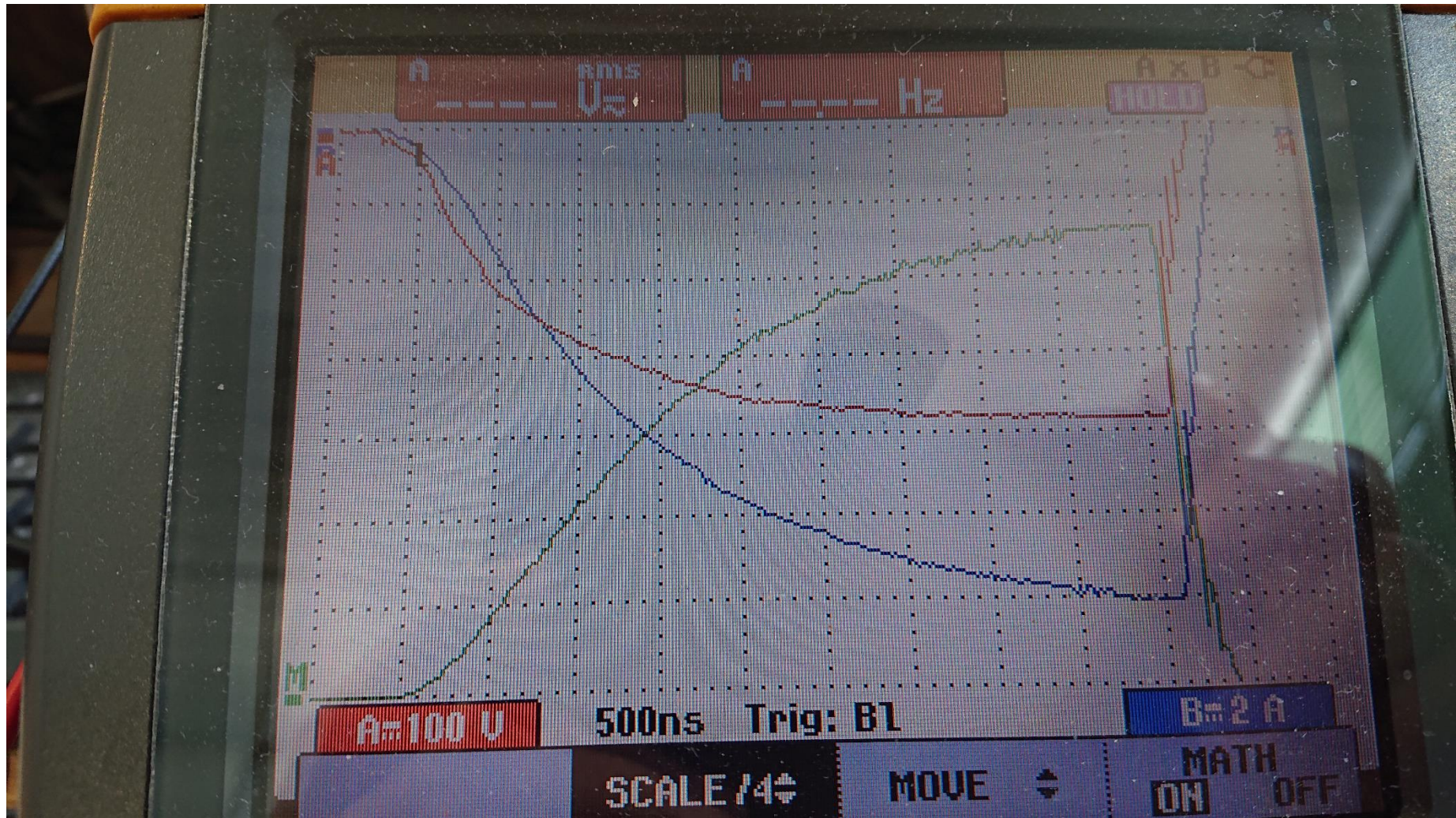
Fig. 6. Snapshot of transversal pulse. Time duration 5\ \mu\text{s} , repetition rate 5\ \text{kHz} . Time division: 500\text{ns} . Longitudinal voltage along the Constantan is in red colour ( 100\text{V}/\text{div} ). Current is in blue ( 2\ \text{A}/\text{div} ), Power is in green ( 800\ \text{W}/\text{div} ). Because inductive effects, the power reached top values only for about 500\ \text{ns} .
