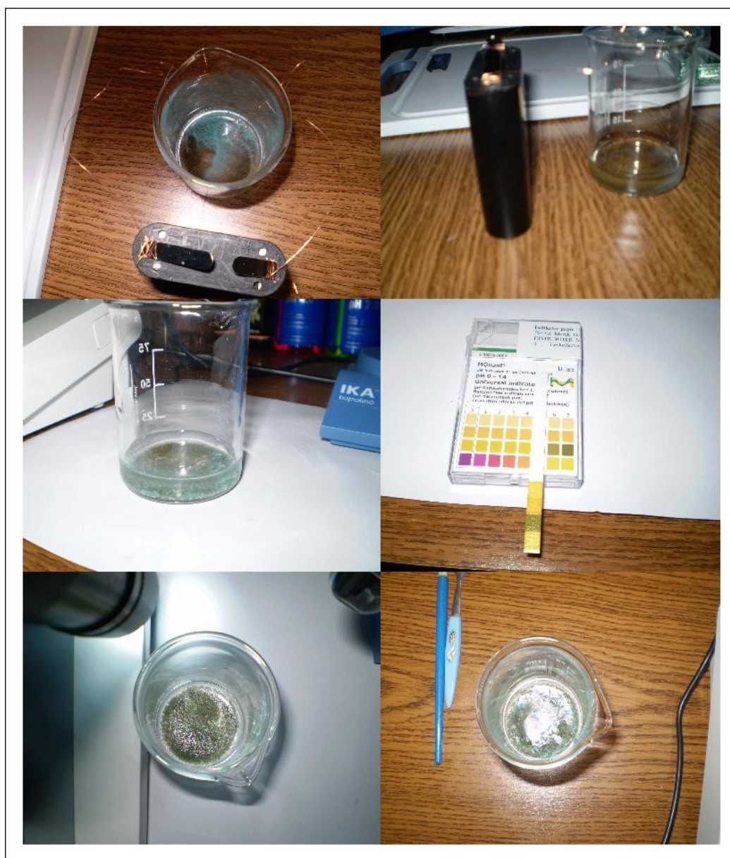
5.4.7.4.3 Figure 349: Electrolysis tests of brown algae in river and distilled water
