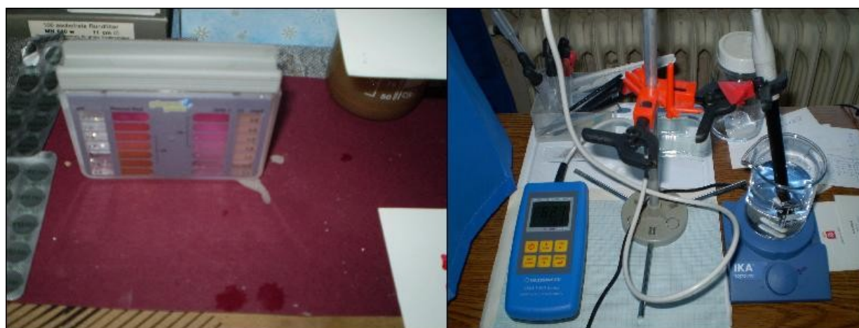
5.5.4.1.4.3.2 Figure 450: Assessment of chlorination and salinity in soil decantates
