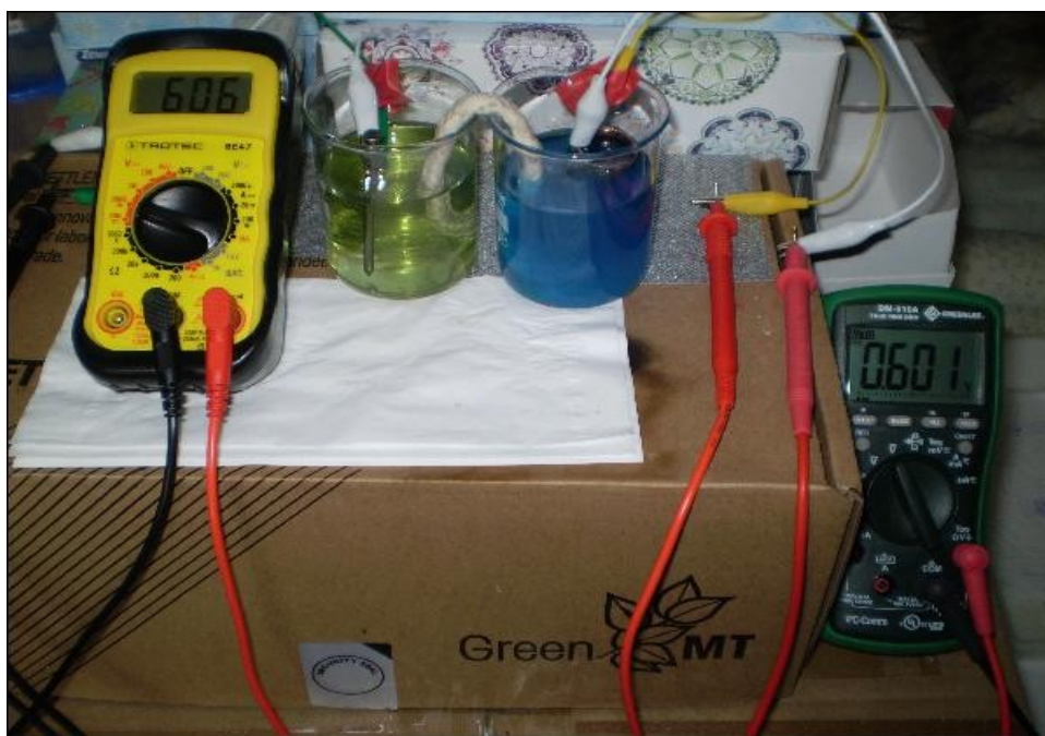
5.4.7.8.9.6 Figure 434: Galvanic cell with saturated solutions of \text{FeSO}_4 \cdot 7\text{H}_2\text{O} and \text{CuSO}_4 \cdot 5\text{H}_2\text{O}
