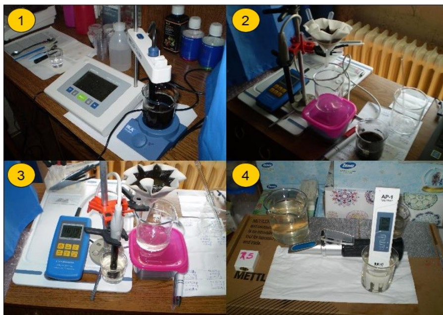
5.5.4.1.1.3 Figure 435: Measurements of pH, conductivity, hardness, and density of humus soil
