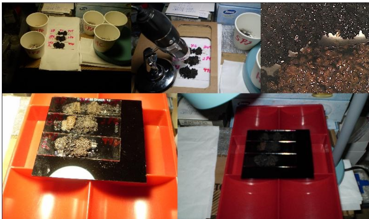
5.5.4.1.4.2.1 Figure 448: Technique for evaluating optical blackness between HC soil and other soils
