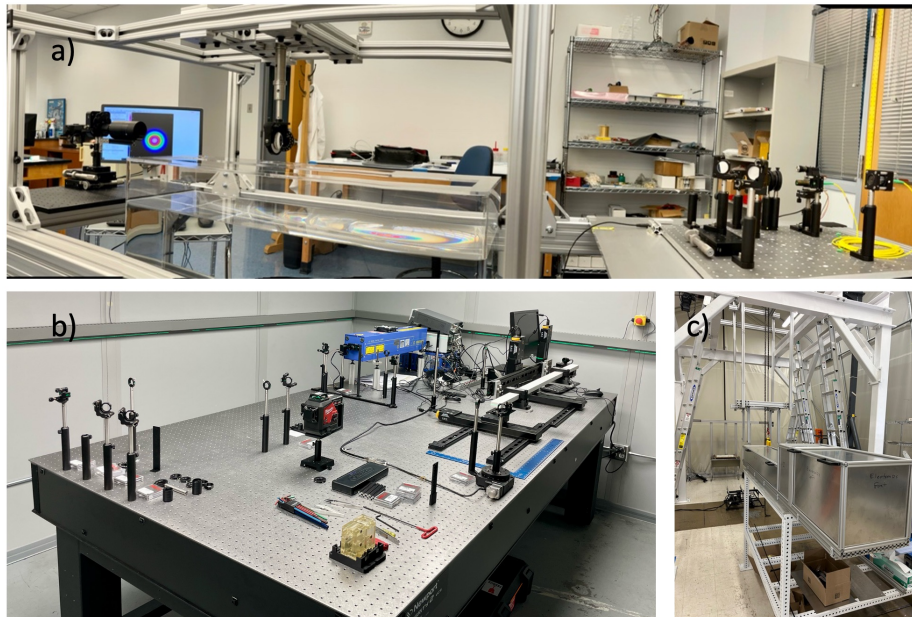
Figure 8.117: Photos of available setups developed during the hpDIRC R&D program that will be used for future QA of 3-layer lenses with laser setup at ODU (a), bars and other optics at Jefferson Lab (b) and readout chain including sensors and electronics and other hpDIRC components in hpDIRC prototype at CRT at SBU (c).
