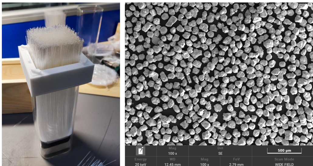
Figure 8.158: Matrix of scintillating fibers prepared to build production FEMC blocks and SEM image of tungsten powder.
