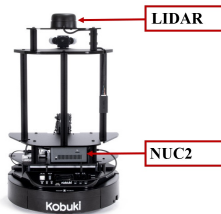
Fig. 1: LoCoBot structure with highlighted sensing module (LiDAR) and computational unit (NUC).
