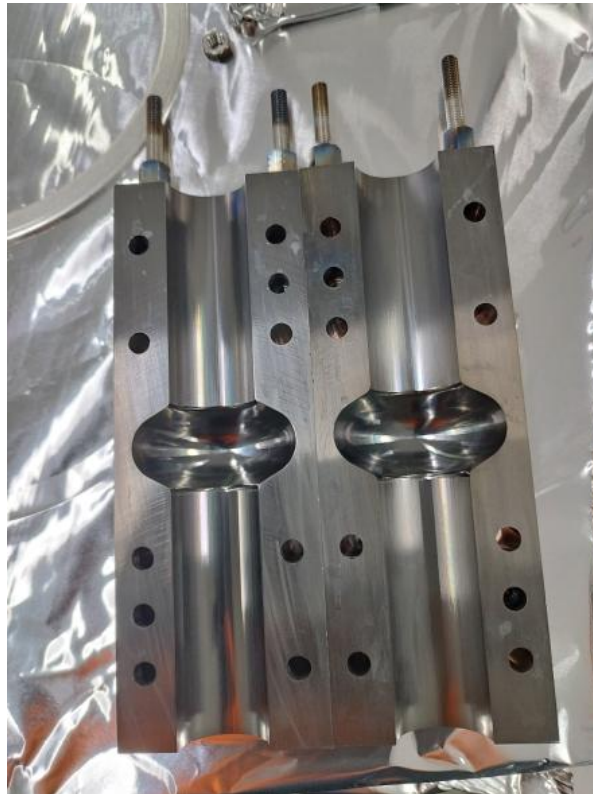
Figure 24. Two coated cavity halves, open for inspection prior to installation in the vacuum system.
