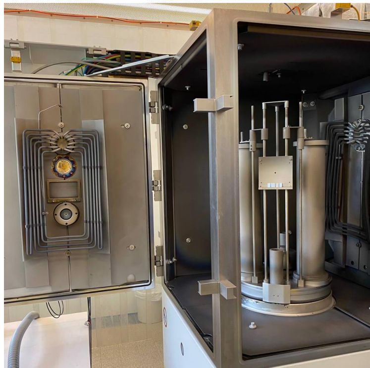
Figure 7. Industrial coating system CC800/9 (CemeCon).
