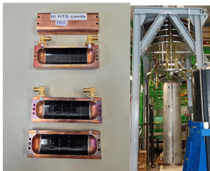
Figure 1. Left: two-segments cavities for axion detection. Right: assembly in the SM18 dipole.
