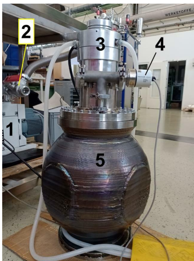
Figure 71. Overview of setup used for Vacuum Test 01. (1) Mechanical (roughening) pump; (2) shut-off valve; (3) turbomolecular pump; (4) vacuum gauge; (5) demonstrator
