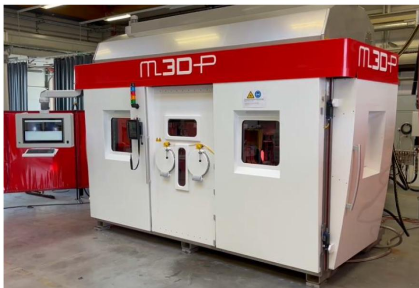
Figure 61. M3DP machine, manufactured by SBI GmbH and used for additive manufacturing activities covered by the HVac project at RHP.
