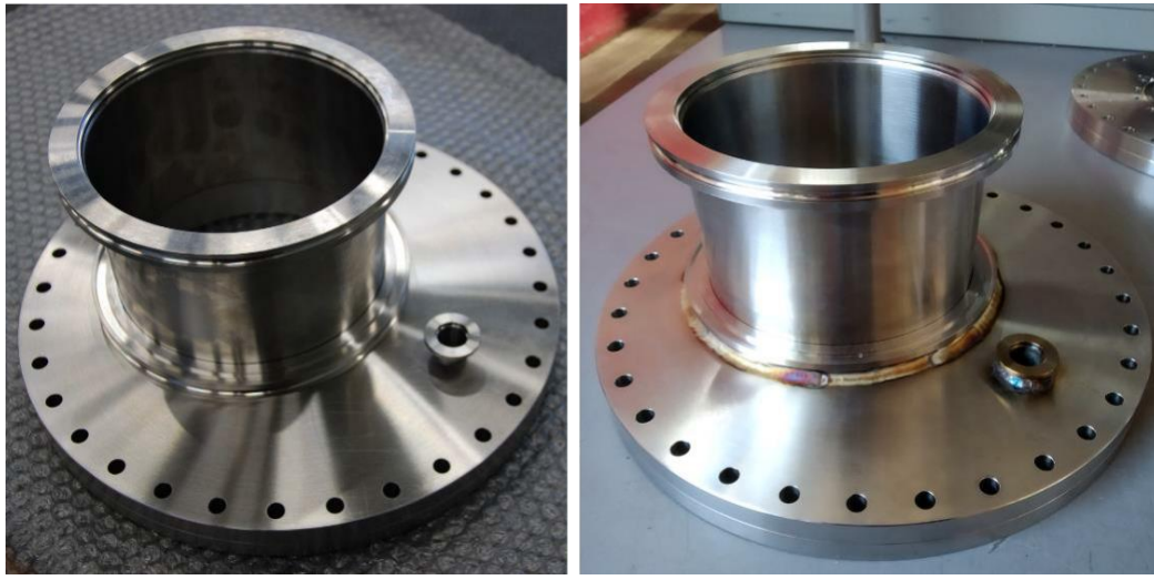
Figure 66. Adaptor used for Vacuum Test 01, performed in-house. Left: blind flanged machined with full and half nipples positioned accordingly. Right: final adaptor after welding
