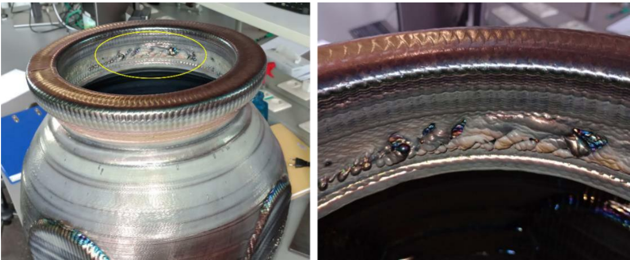
Figure 69. Left: material deposition inconsistencies indicated at the interior portions of the upper flange; right: closer look at the defects
