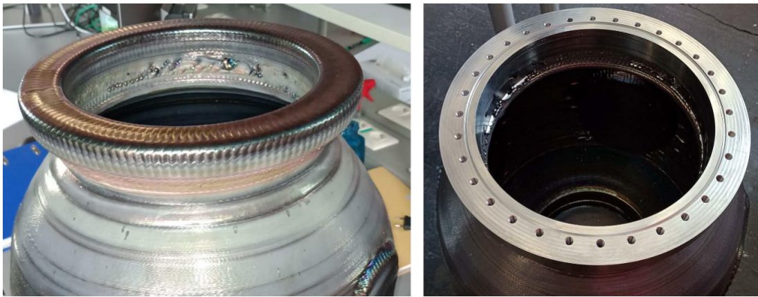
Figure 65. Vacuum chamber demonstrator before (left) and after (right) post-processing milling operation. Flange size correspond to standard DN250CF.
