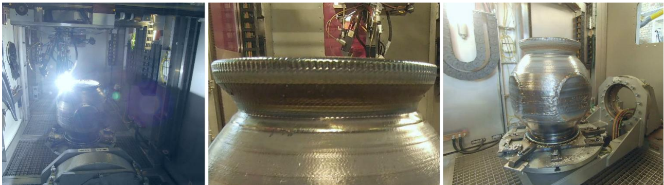
Figure 64. Pictures of the PMD process during the manufacturing of the upper flange section. From left to right: beginning of the upper flange section being printed; final upper flange section, showing the ramp-like shape used to support the upper flange; final look of the entire chamber in the as-printed condition
