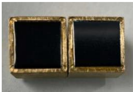
Figure 4. samples of large-size HTS tapes, prepared at ICMAB for RF characterization with the 8 GHz dielectric resonator
