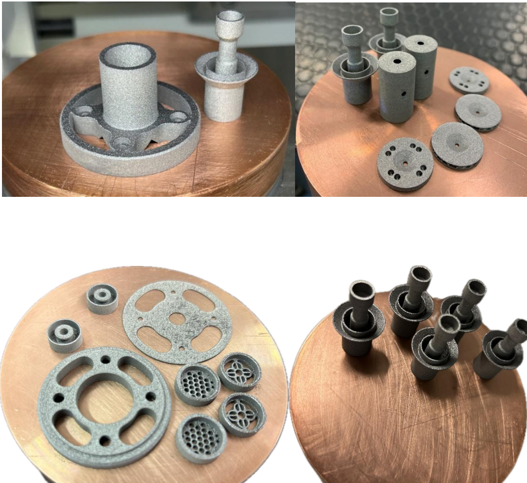
Figure 37. Set of photos of the FEBIAD-type ionization source components and the Thermionic emission test setup additively manufactured in Ta at the DIAM lab.
