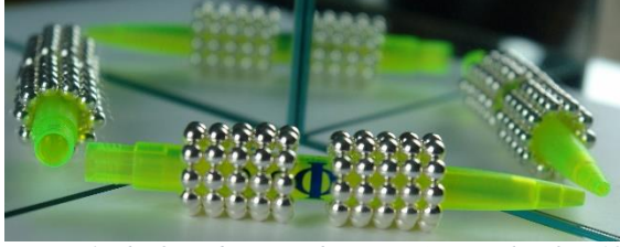
Figure 4. The force between these two S=5 stacks of L=10 rings decreases with a power of -22 .
