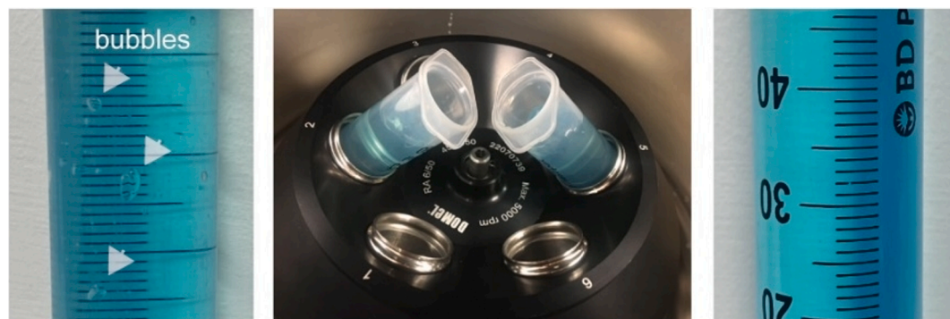
Fig. 12. Effect of a degassing procedure on aqueous gel. Example of aqueous gel prior to (left), and after (right) centrifugation. Alternatively, the syringes can be placed in a vacuum chamber for degassing.
