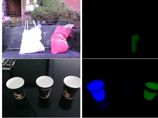
Fig. 4. Two examples of images used in the test. On the left are the standard images, and on the right are thermal images mapped according to the ThermalSense algorithm (blue is hot and green is cold).
