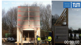
Unprotected GLT ceiling, walls with 1 x 18 mm gypsum plasterboard
