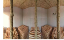
Unprotected GLT ceiling, walls with 1 x 18 mm gypsum plasterboard
