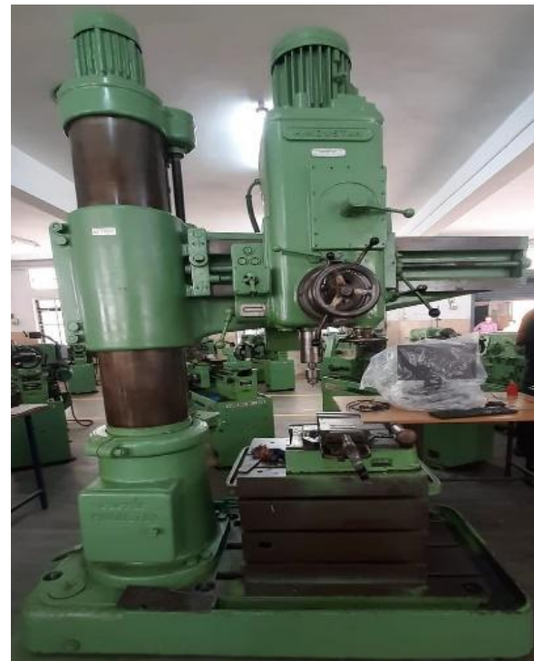
Fig. 3: Radial Drilling Machine
