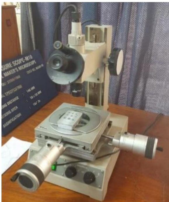
Fig. 6: Tool Maker's Microscope
