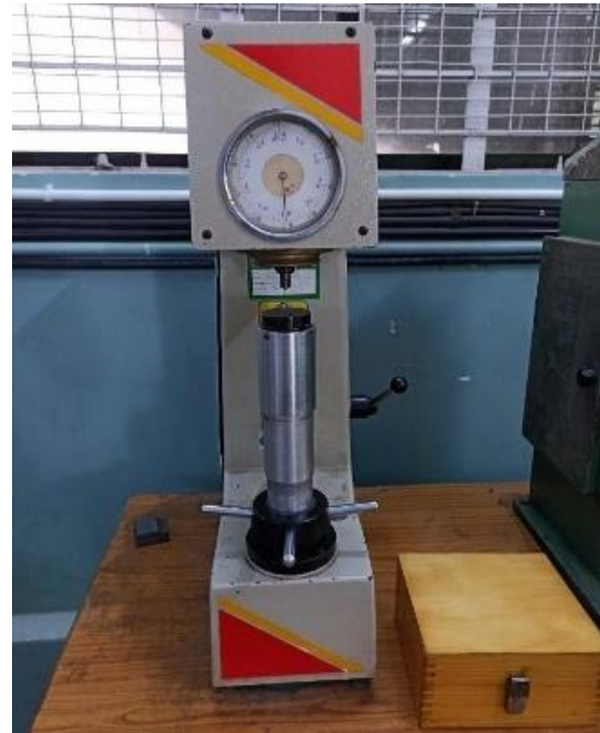
Fig. 2: Rockwell Hardness Testing Machine
