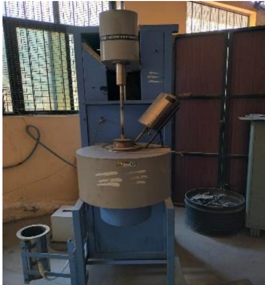
Fig. 1: Stir casting process
