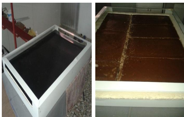
Fig. 2: Absorber plate in contact with paraffin wax
