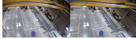
Fig. 2. Video frame showing the distortion correction using the intrinsic calibration parameters of the camera lens and the resulting undistorted image.
