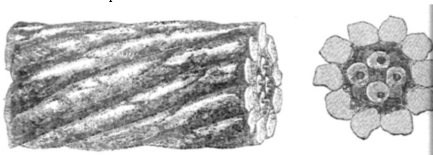
PIECE OF 1851 CHANNEL CABLE PICKED UP LATER.
