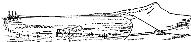
LANDING THE SHORE END FROM A TELEGRAPH SHIP.
