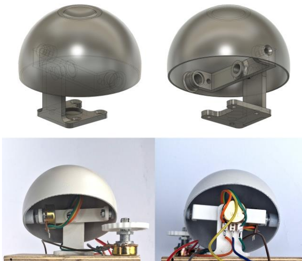
Figure 2. 3D model and an actual view of the dome-shaped joystick component
