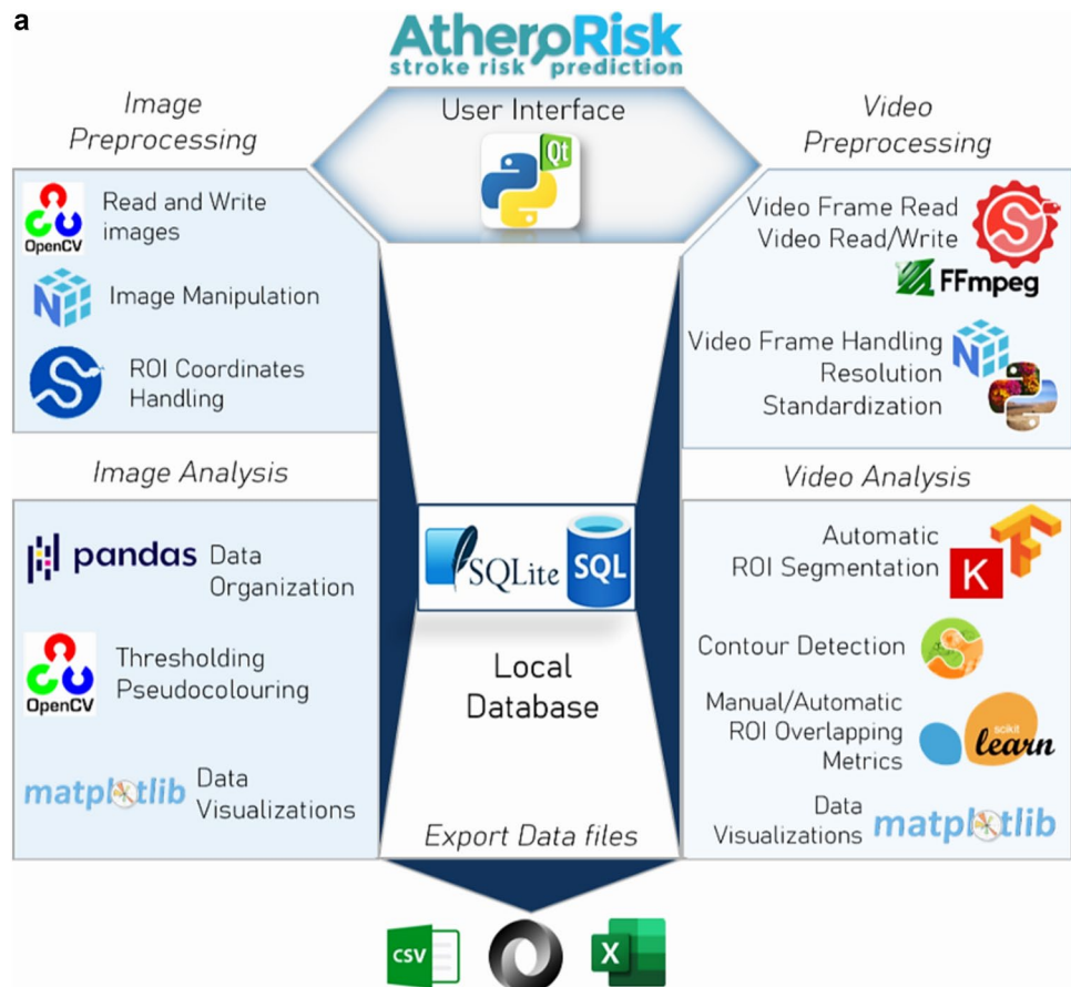
Fig. 1 a The class flow diagram for the first version of the AtheroRisk software as proposed in this study for carotid plaque processing and analysis in B-mode ultrasound longitudinal images and videos, b High-level architecture of the AtheroRisk software incorporating all the proposed software packages. ROI region of interest
