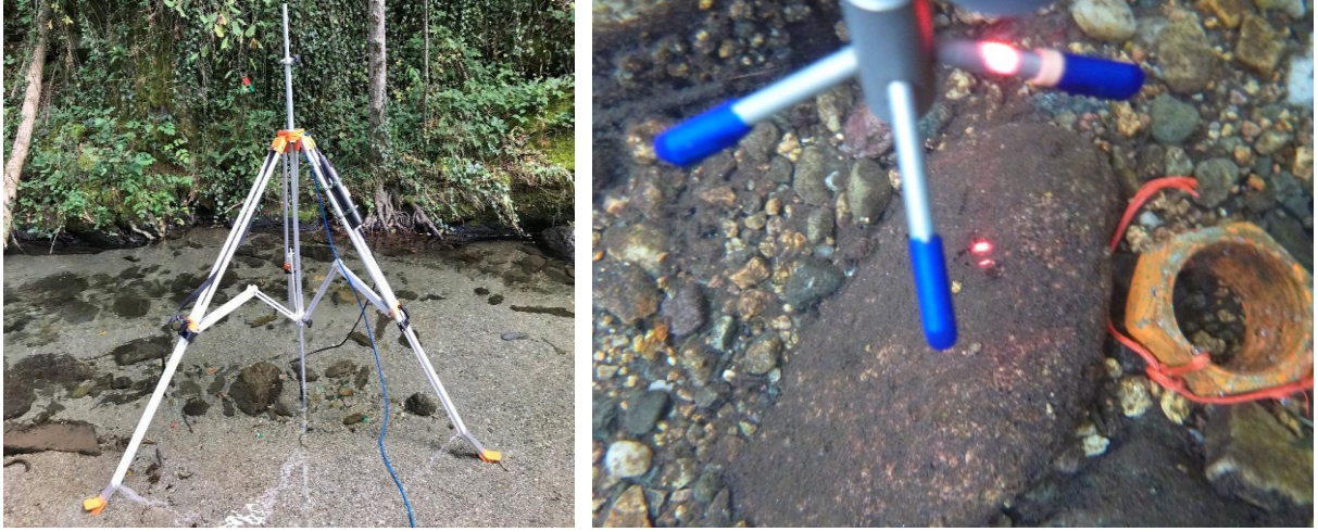
Fig. 2. Left, holding frame for ADV (section 5.2.1) adapted from a tripod for a total station, with attached Vectrino Profiler (Nortek AS, Norway) measuring high-frequency flow velocity at 2 cm above the stream bed. Custom made for RESTOLINK. Right. Underwater photos of the sampling location are marked with a metal nut and a laser pointer indicating the precise sampling spot.
