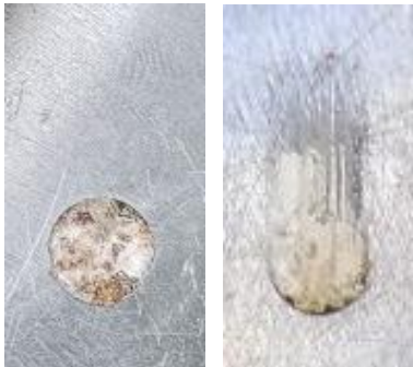
Figure 13 Crushed sand fragments and scratch marks on the lower lateral moving plane.
