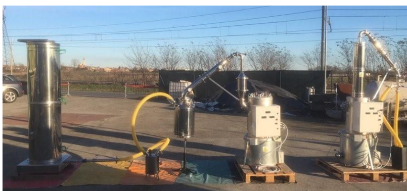
Fig.33: Converting Marine Litter with Pyrolysis System
