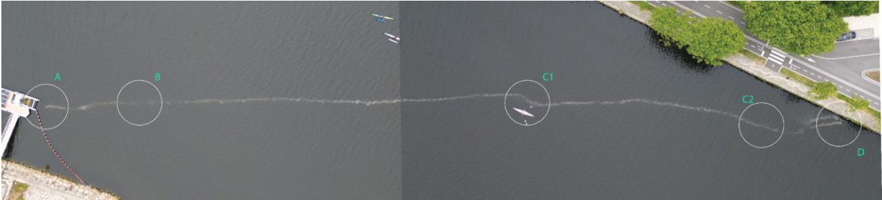
Figure 4.8 - Technical assessment of the Bubble Barrier in Vila do Conde after the optimization. Indicated are points of interest: (A) section at the Catchment System (B) weaker part of the Bubble Barrier (C1,2) curves (D) exposed extremity. Important note: As photos are only a snapshot, one should be cautious to draw conclusions based on a single photo.
