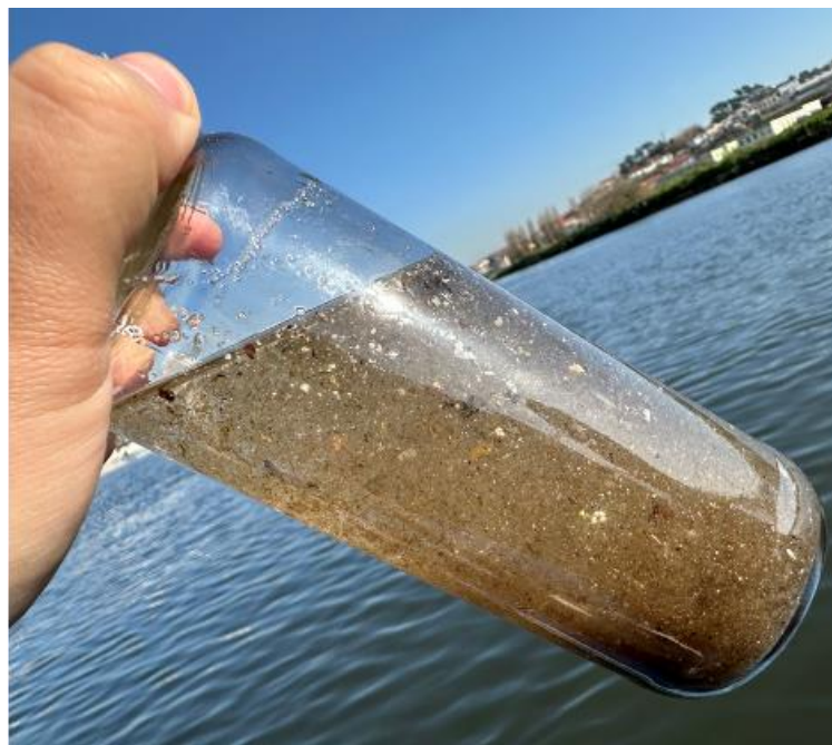
Figure 6.10 - MP sample collected in the bubble curtain with the manta net.
