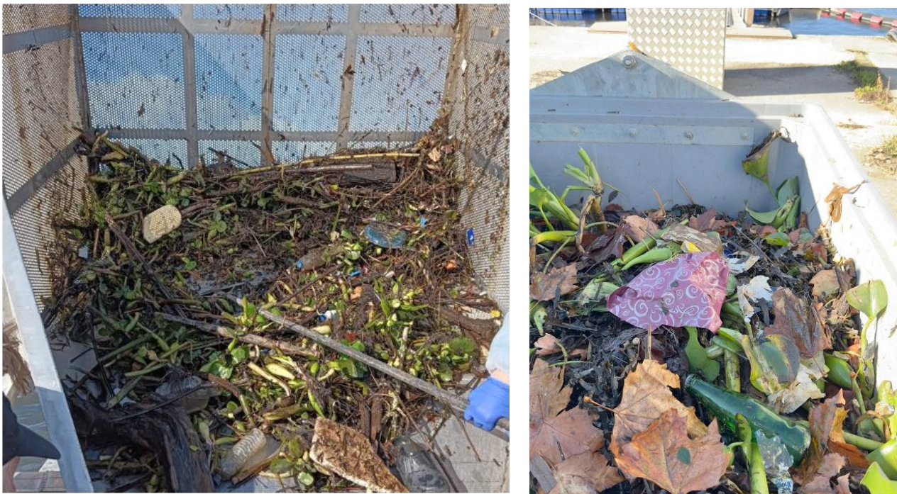
Figure 6.14 - Emptying the catchment system and collected litter for classification.
