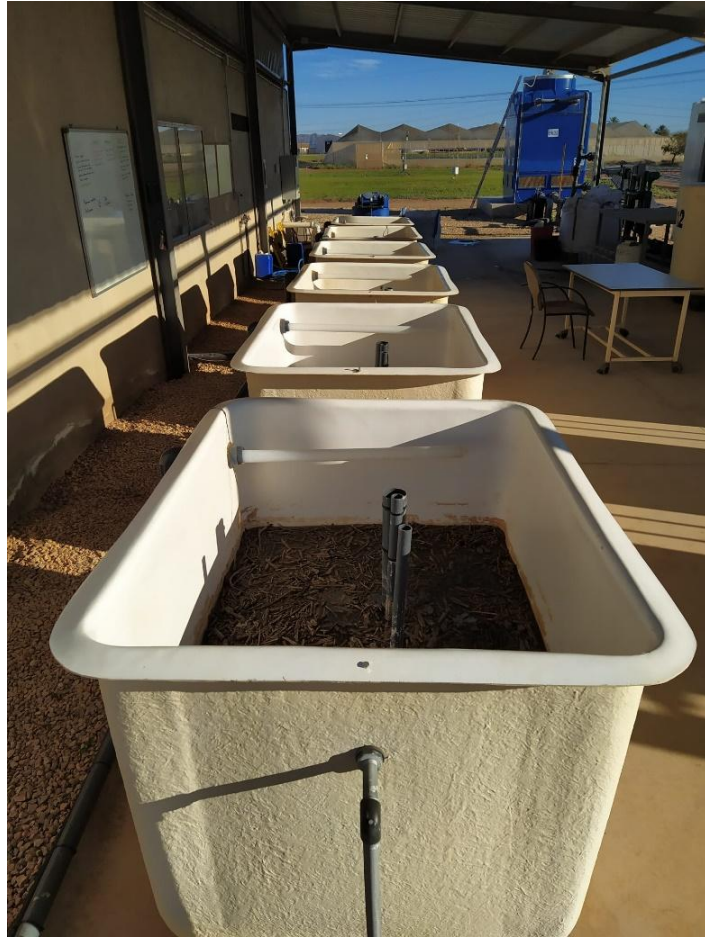
Figure S1. Citrus woodchip bioreactors in the pilot plant at the Agri-food Experimental Station Tomás Ferro (ESEA) of the School of Agricultural Engineering, Technical University of Cartagena (ETSIA-UPCT) to denitrification experiment with brines.
