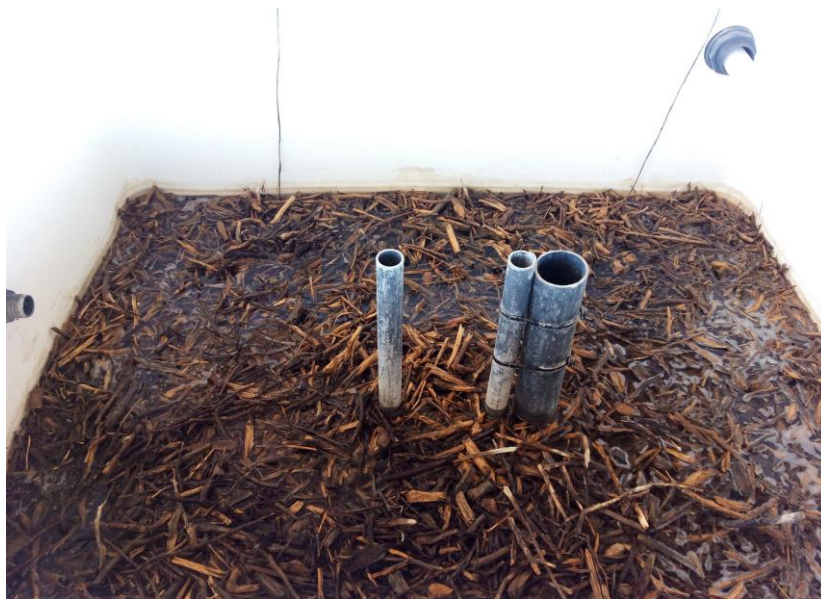
Figure S2. Citrus woodchips placed in a bioreactor in the pilot plant at the Agri-food Experimental Station Tomás Ferro (ESEA) of the School of Agricultural Engineering, Technical University of Cartagena (ETSIA-UPCT) to denitrification experiment with brines.
