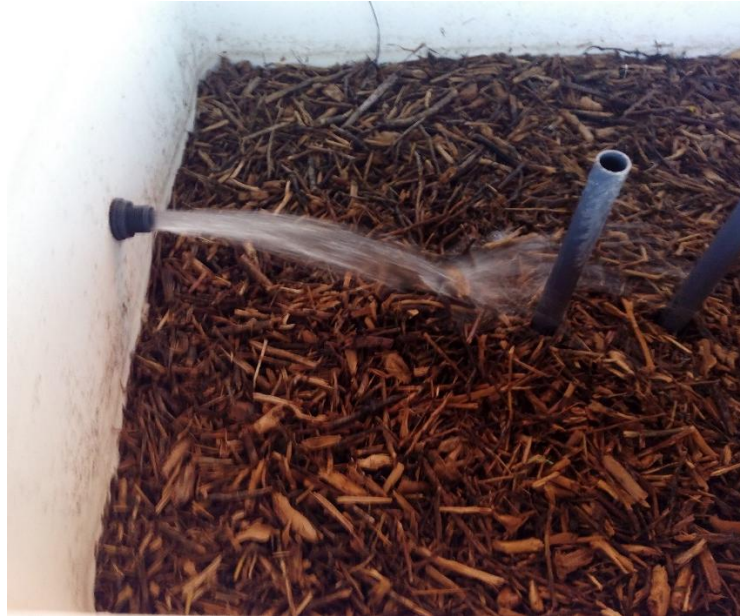
Figure S3. Method of introducing the brine in the bioreactor in the pilot plant at the Agri-food Experimental Station Tomás Ferro (ESEA) of the School of Agricultural Engineering, Technical University of Cartagena (ETSIA-UPCT) to denitrification experiment with brines.
