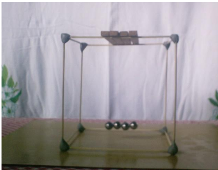
Figure 13:– Apparatus built with steel balls, fishing line, wood, barbecue skewers (to support the suspended balls), superbonder glue and caulk.
