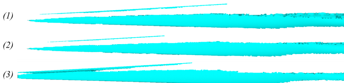
Figure 13: topology optimisation results: 1 – CFD; 2 – uniform pressure; 3 – point load
