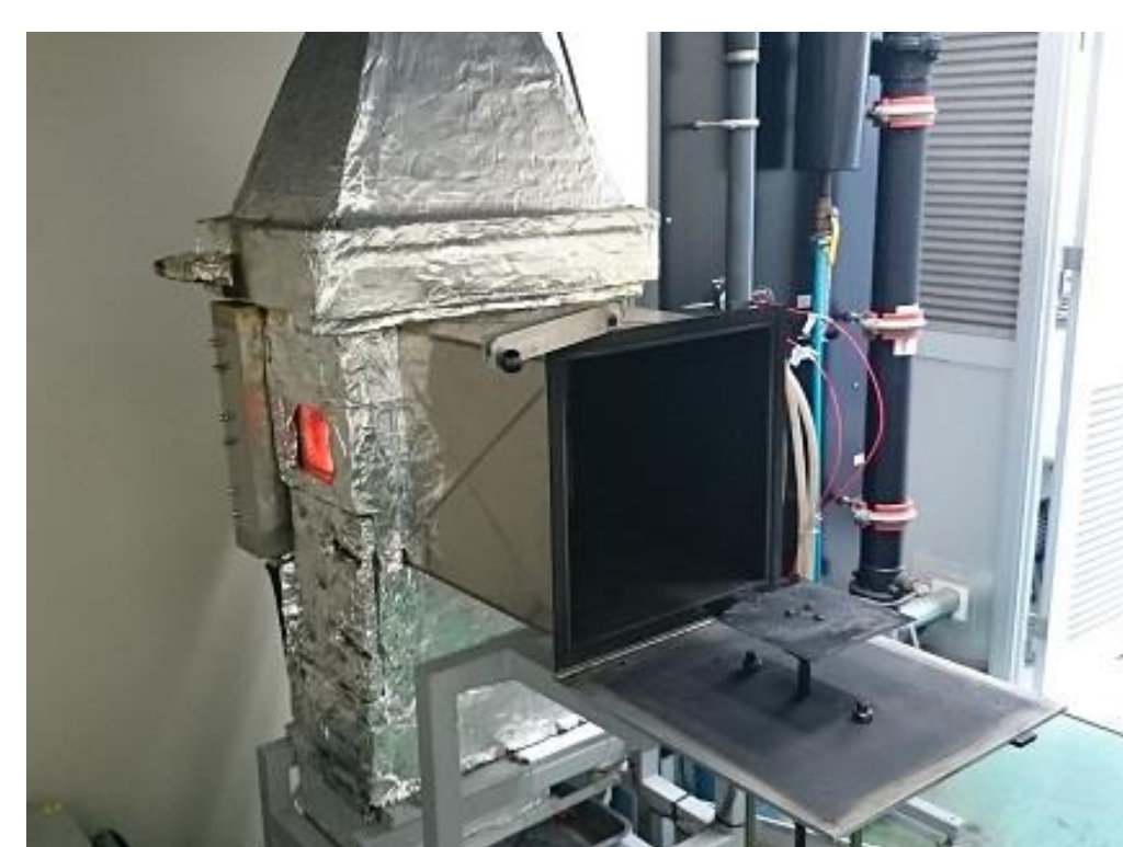
Figure : Maximum heat release rate during fire test and total heat release at two minutes of thermoplastic and thermosetting composites (Left), A fire instrument for OSU-HRR (Right).
