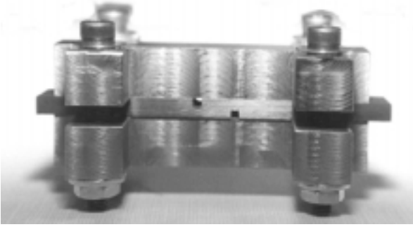
Fig. 1. The double notch shear testing setup.
