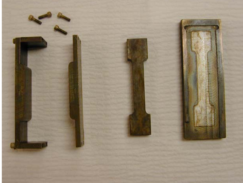
Figure 2 Photograph of The Steel Mold
