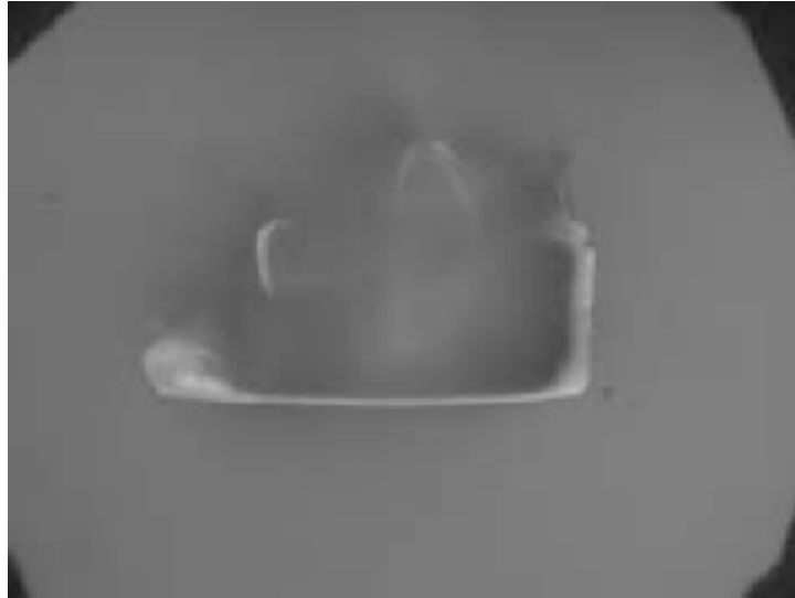
Fig. 10: Element of micro-gear fabricated by the photopolymerization process.
