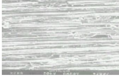
Fig 5 Fractograph for T300/3261 composites
