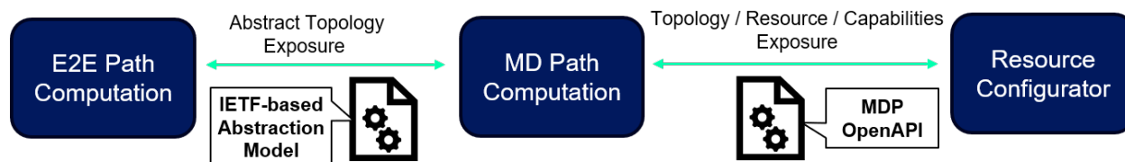
Figure 2-4. Information models exchange in support of E2E Topology Exposure
