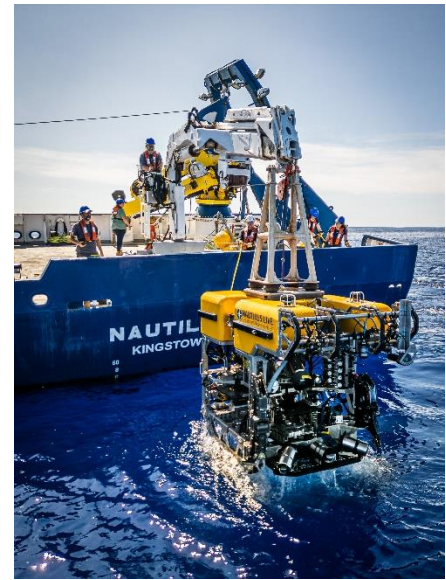
The Ocean Exploration Trust at work, recovering the Hercules ROV from the Nautilus. Photo provided by the speakers.
