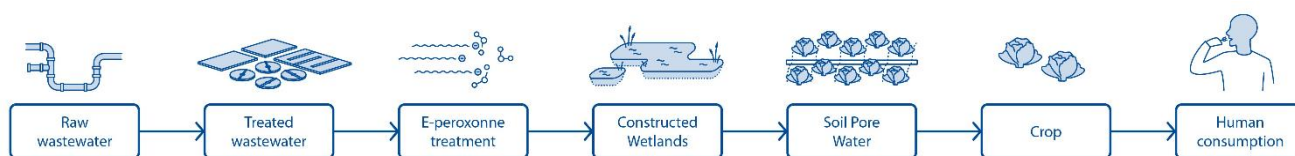
Figure 2. Technological treatment train for water reuse for agricultural irrigation (Source: KWB)
