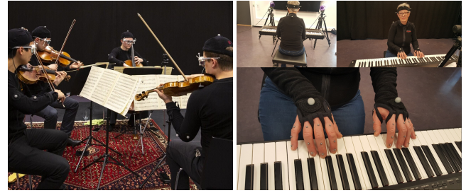
Figure 4: The left image shows musicians playing violin, motion captured using an optical MoCap system with reflective markers, tracking their body and instrument motion (image extracted from [Fut]). The right image shows a musician playing piano, while the movements of the finger joints are tracked with 5mm reflective markers (image extracted from [Ger]).
