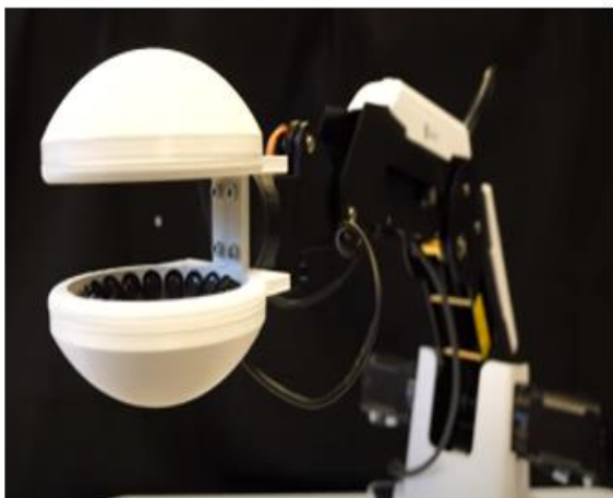
Figure 1: Basic acoustic levitation setup with transducer, reflector, and levitated object
