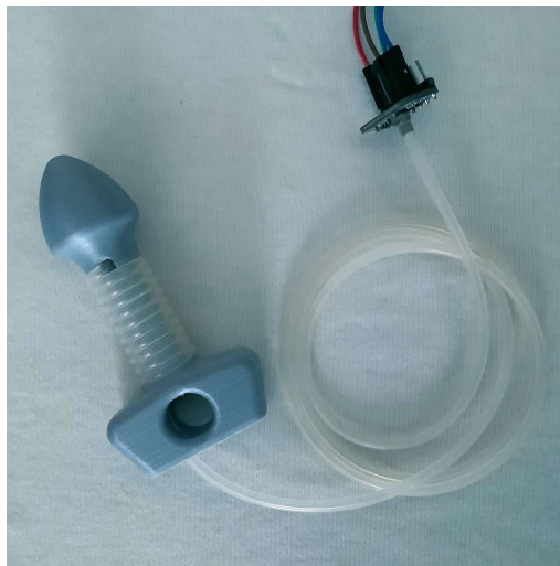
Fig. 2. Anal Probe with Pressure Sensor.
