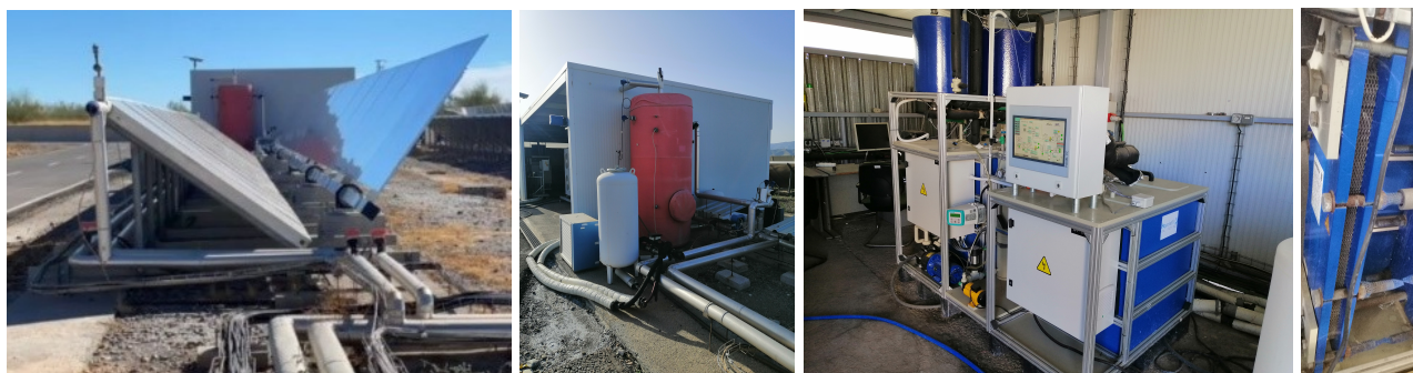
Figure 1: The PSA setup includes the solar thermal field, the thermal storage tank, the MD unit, and the heat exchanger.
