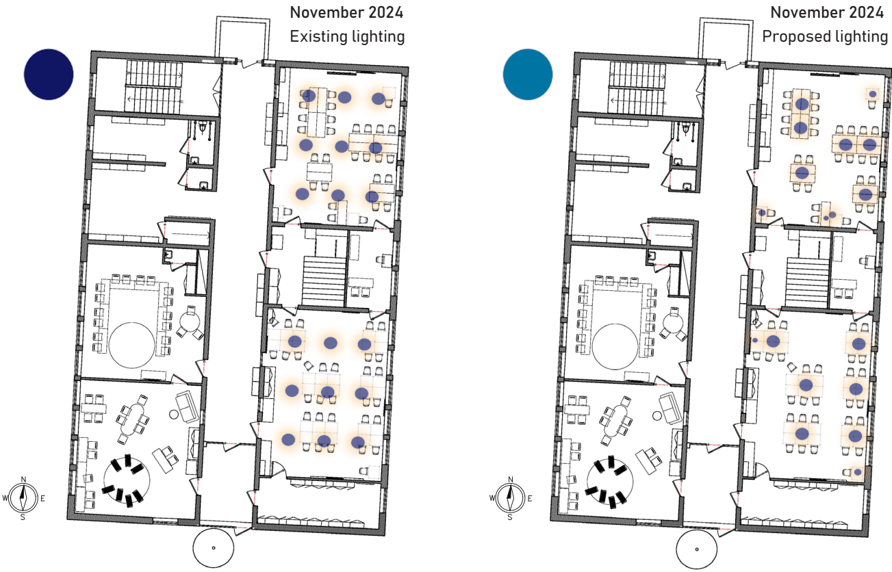
Figure 4: The left floor plan illustrates the existing placement of lighting. The right floor plan is a proposal on how lighting can be placed based on the furniture configuration.
