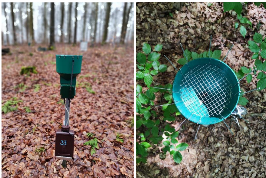
Fig. S2: Throughfall sampler from the front and from above.
