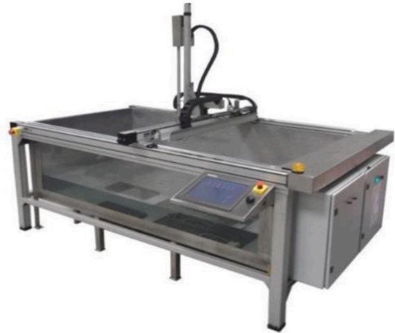
Fig. 5. Phased array inspections - Immersion tank.
