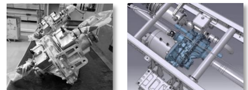
Figure 6 Transfer Box installation
