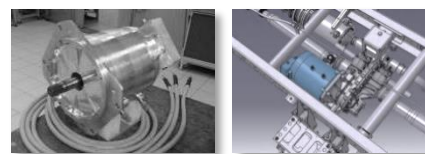
Figure 7 E-Motor Installation
