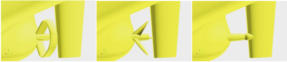
Figure 2. GRIP ESD designs: MARIN BSD (left), HSVA Pre-Swirl Stator (middle) and VICUS Rudder Bulb (right)
