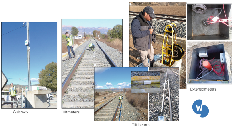
Fig. 9. IoT devices installed on the FGB railway track as a part of ICOS Railway Use Case
