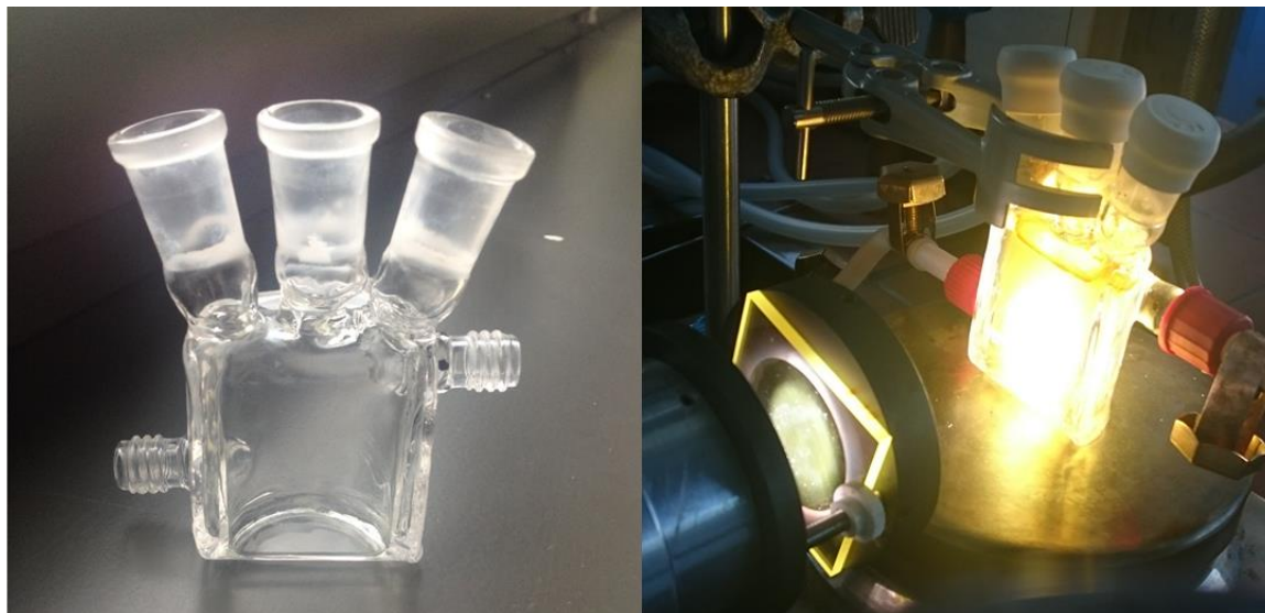
Figure S13. Photos of the reactor (left) catalytic reaction setup (right).
